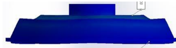
Figure 13. Stress Result of YMMotor Cover Side View
